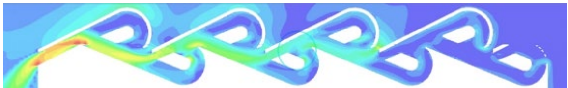
Figure 1. CFD Visualization of Directional Flow and Velocity Distribution through a Tesla Valve Geometry
